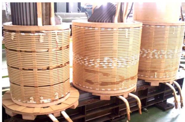
Fig. 10 HV and LV winding coil
