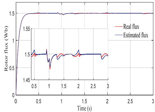
Fig. 7. Estimated and real rotor flux during step change of reference speed
