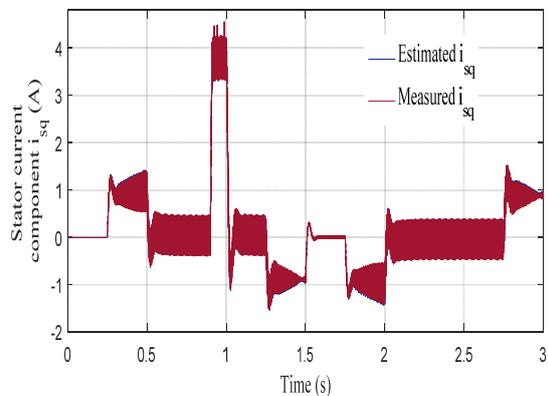
Fig. 9. Estimated stator currents evolution during step change of reference speed
