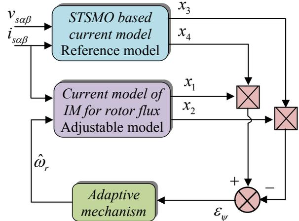
Fig. 3. Classical Model reference adaptive scheme for speed estimation
