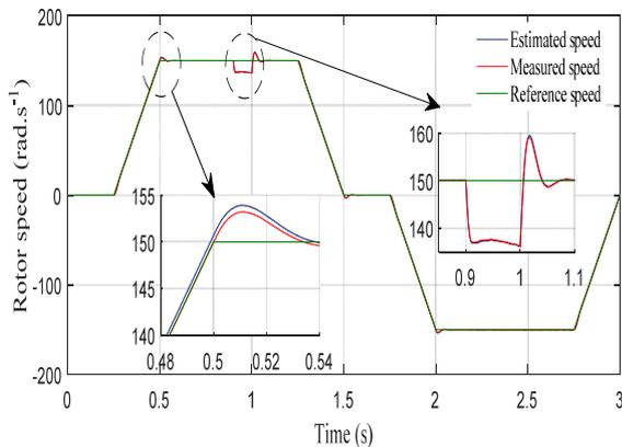
Fig. 5. Response of the system at free acceleration test. The reference, actual and estimated speed.
