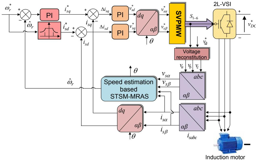
Fig. 4. Classical Model reference adaptive scheme for speed estimation
