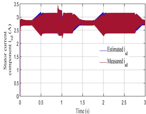
Fig. 8. Estimated stator currents evolution during step change of reference speed
