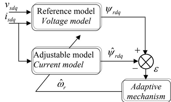
Fig. 1. Rotor speed estimation based on MRAS structure
