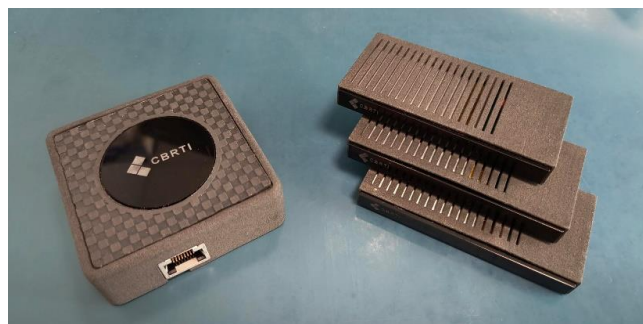
Fig. 2. Author's coupling solutions created in the project – actual prototypes of the UWB anchor (left) and UWB tags (right)
