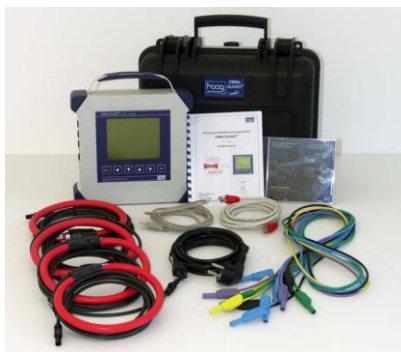
Fig.2. Omni-quant instrument for power quality measurements
