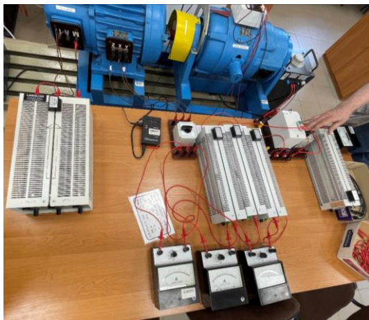
Fig. 1. Physical implementation of the concept of a station for recording acoustic signals for selected pre-failure states of an electrical machine
