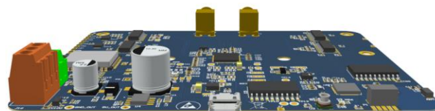
Fig. 2. 3D visualization of the printed circuit board of a hybrid tomographic probe
