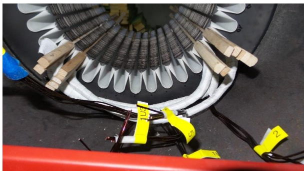
Fig.6. Winding stator coils made by enamelled copper wires
