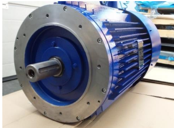
Fig.7. Finished double-voltage double-speed induction motor P_n=50/8 kW, n_s=3\ 000 / 1\ 500 rpm to drive a fan
