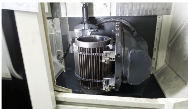
Fig.5. Machining of the motor enclosure
