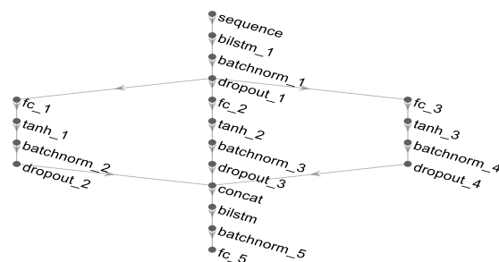
Fig.4. Branching structure in a multi-branch neural network
