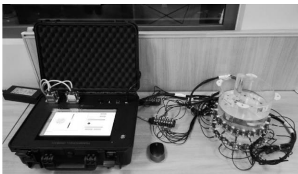
Fig.1. Tomograph with a test tank and settings: excitation frequency 10kHz, excitation current 1mA, number of sampling periods 3. Number of measurement electrodes 32. Configuration of measurement electrodes 2x16. 2.5D measurement sequence.
