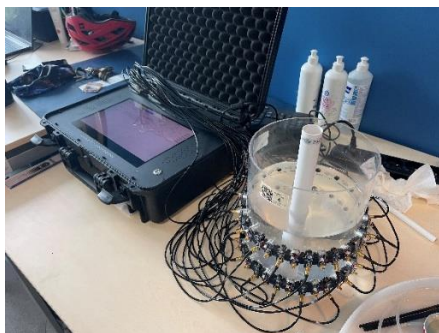
Fig. 1. The measurement setup – a physical model of an industrial reactor connected to a hybrid EIT/ECT device
