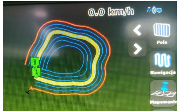
Fig. 3. Traces of travel along the A-B curve line recorded by navigation
