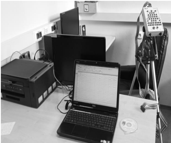
Fig.1 Mitsar 202 recording equipment with a computer [source: own]
