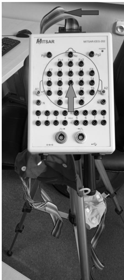
Fig.2 Mitsar 202 recording apparatus [source: own]
