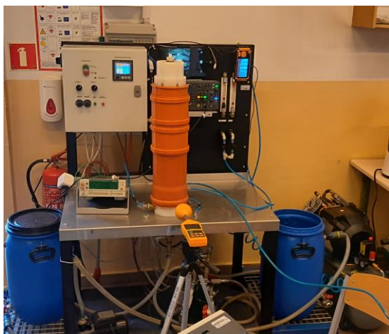
Figure 1. View of the laboratory bench equipped with a cold plasma generator with the location of the meter at a height of 10 cm in relation to the structural frame
