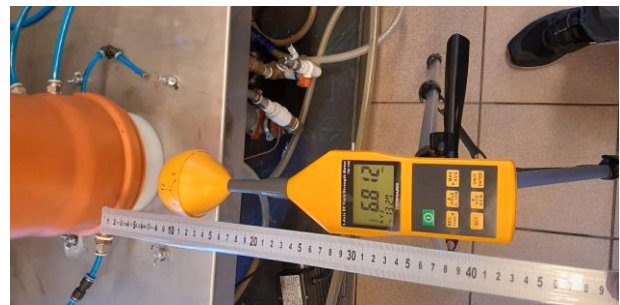
Fig 2. Location of the TM 196 meter in relation to the cold plasma generator.
