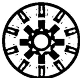
Fig. 1. A 6/4 configuration of switched reluctance motor drive
