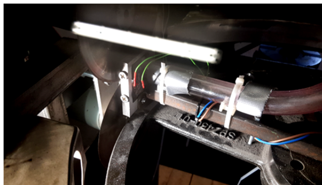
Fig. 4. Cutting unit of the scarification device
