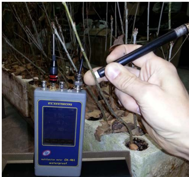
Fig. 6. Measurement of admittance of the shoots of pedunculate oak seedlings using the Elmetron CX-461 universal device
