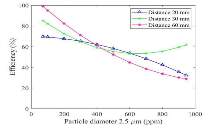
Fig. 11 Efficacy of PM<sub>2.5</sub> dust abatement across diverse electrode spacings.
