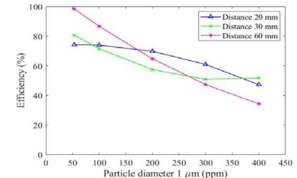
Fig. 10 Efficacy of PM<sub>1</sub> dust abatement across diverse electrode spacings.
