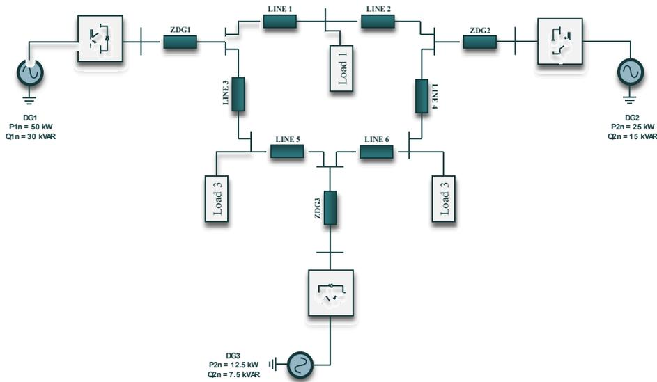
Fig. 3. (3) DGs meshed AC microgrid inspired from IEEE 9 bus test feeder
