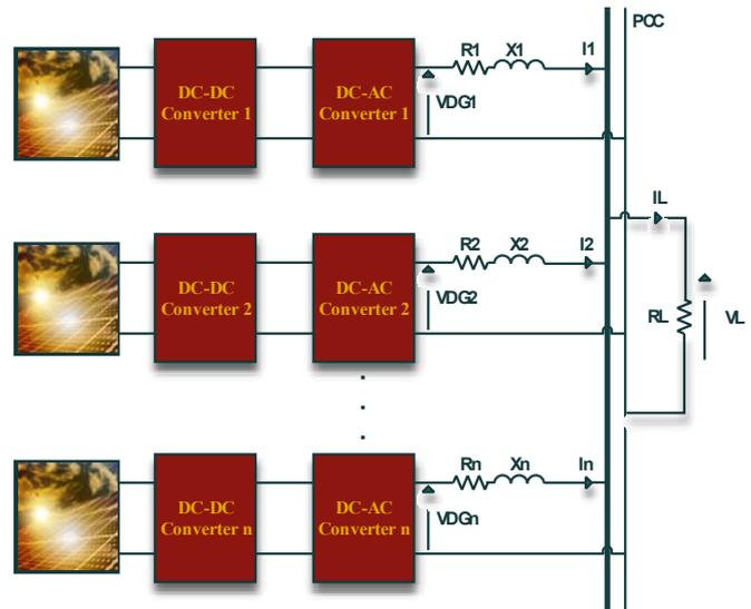
Fig. 1. AC Islanded Microgrid with  $n$  converter
