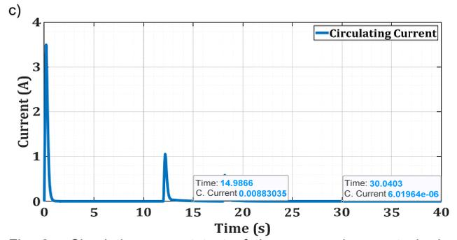
Fig. 9. Circulating current test of the proposed current sharing method. (a) Same transmission lines' impedance value. (b) Different transmission lines' impedance values. (c) Different transmission lines' impedance values with consideration of load variations
