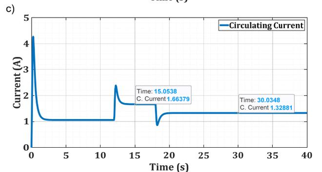
Fig. 7. Circulating current test of the power sharing method in [26]. (a) Same transmission lines' impedance value. (b) Different transmission lines' impedance values. (c) Different transmission lines' impedance values with consideration of load variations
