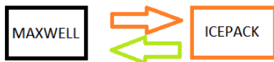
Fig. 4 Scheme of "coupling" in the process of calculating the bar temperature (two separate programs calculating the bar temperature)
