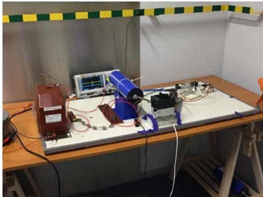
Fig.3. A picture of a laboratory model of a device for destroying Flash memory .
