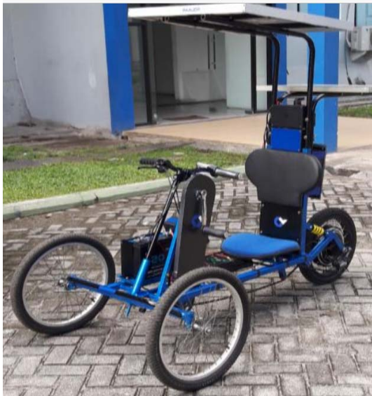
Fig. 3. Designed three-wheeled electric bicycle
