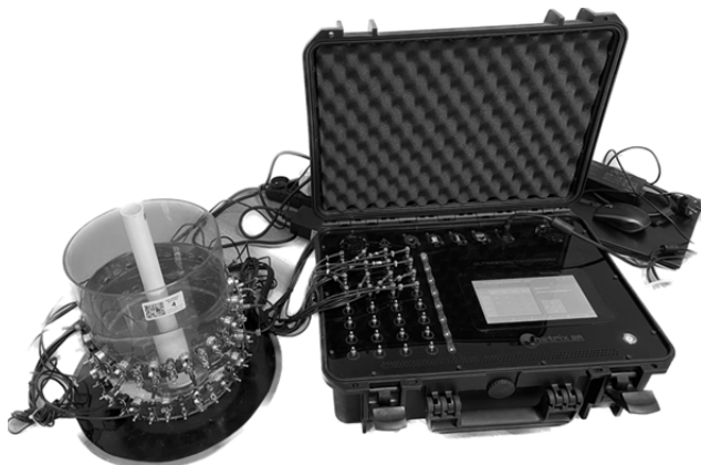
Fig.1. Physical model for validation of image reconstructions based on UST measurements.
