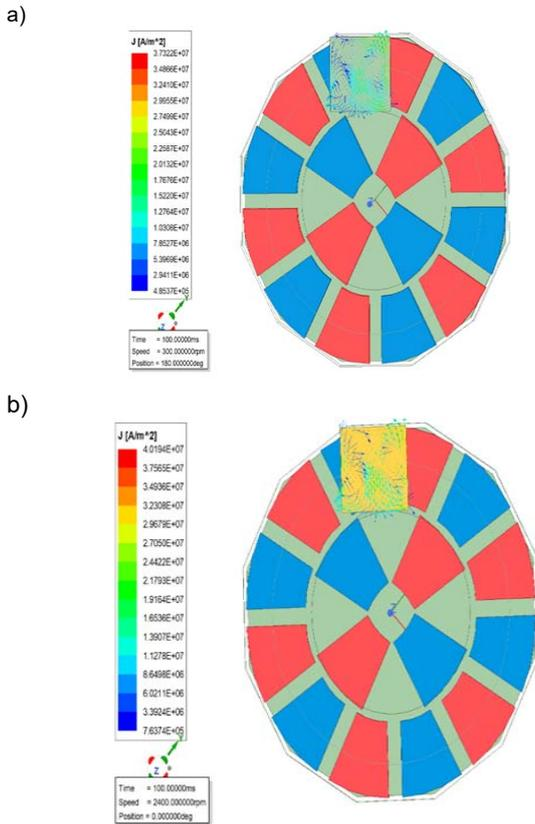
Fig. 4 Eddy current in 3D rectangular copper particle: (a) 300 Rpm, (b) 2400 Rpm
