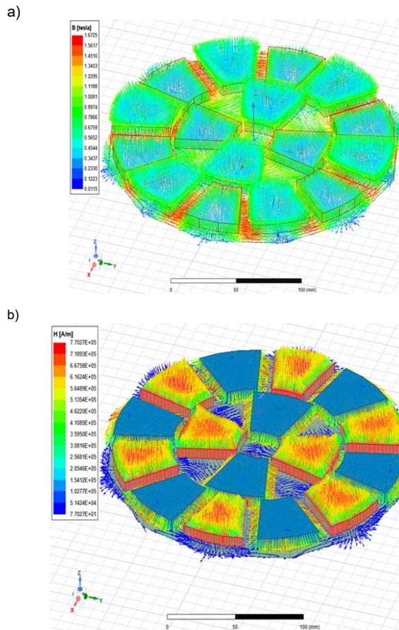
Fig. 3 Magnetic characteristic of separator: (a) Magnetic flux density norm (T), (b)Magnetic field
