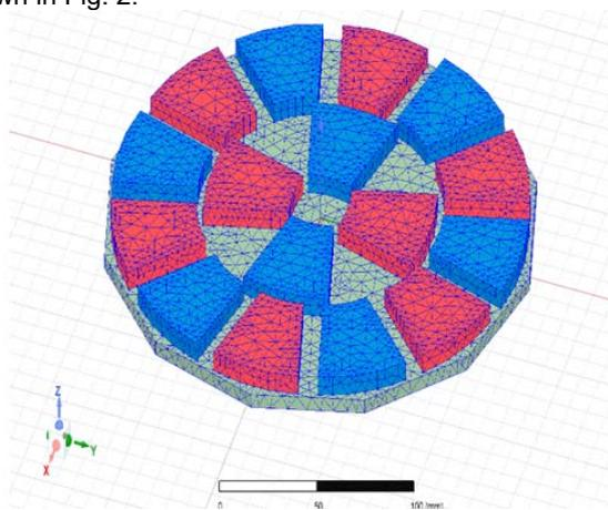
Fig. 2 Mesh of magnetic disk
