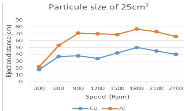
Fig. 8 Ejection distance of non-ferrous particles
