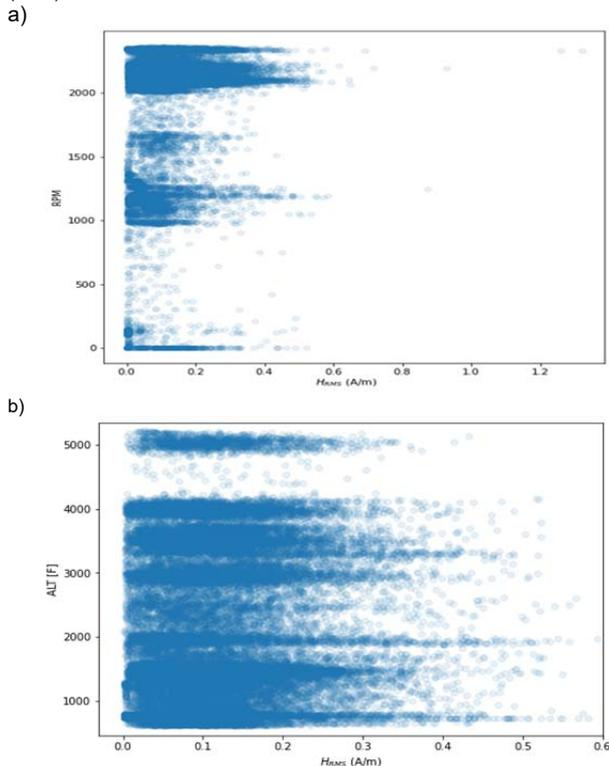
Fig.8. The dependence of the magnetic field of flight above 100f in the Tecnam P2006T aircraft: a) rotational speed (RPM), b) altitude (ALT)
