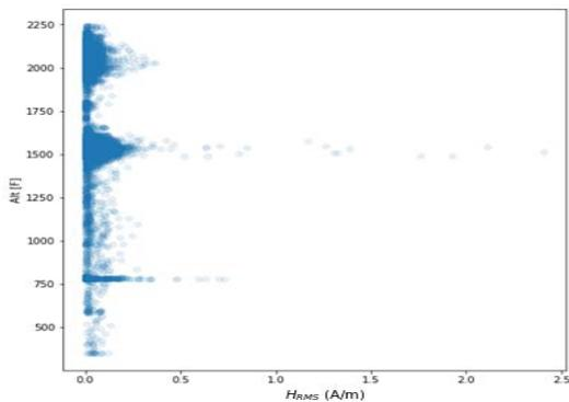
Fig.4. The dependence of the magnetic field on the altitude (ALT) of flight above 100f in the Aero AT3 aircraft
