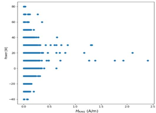
Fig.6. The dependence of the magnetic field in relation to power (power) in the range of 10W during flight at an altitude above 100f in the Aero AT3 aircraft
