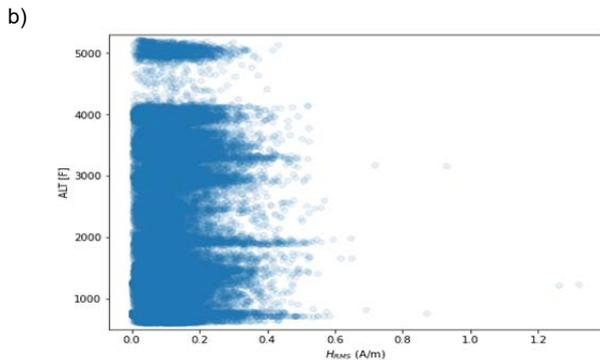
Fig.7. The dependence of the magnetic field on flight parameters in the Tecnam P2006 aircraft: a) rotational speed (RPM), b) altitude (ALT).
