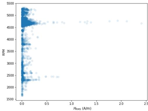
Fig.3. The dependence of the magnetic field on the rotational speed (RPM) of flight above 100f in the Aero AT3 aircraft
