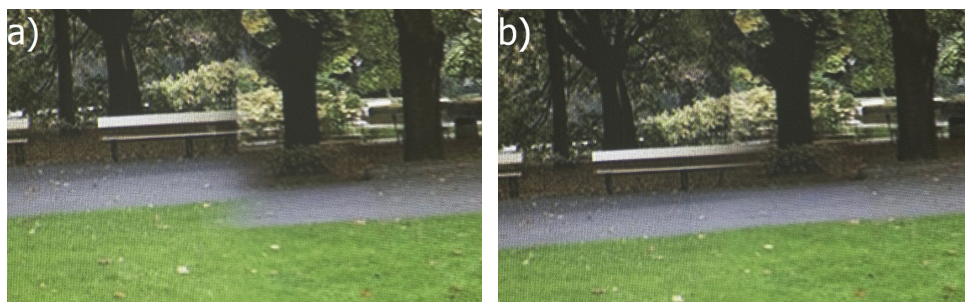
Fig. 3. The consequences of stitching with wrong geometry are visible on the example images of the Warsaw Saski Garden displayed in SEMI-CAVE. a) enlarger detail before correction, b) the same detail after correction of geometry.
