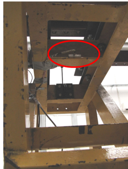
Fig.3. Closest possible placement of the accelerometer on the test stand/test interface (in the red circle, source L-Ilot)
