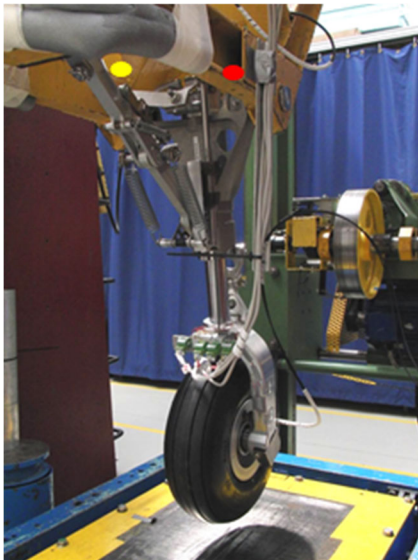
Fig.2. Landing gear mounted to the drop test stand. Force measurement plate is visible under the wheel. (dots: see text, source L-Ilot)
