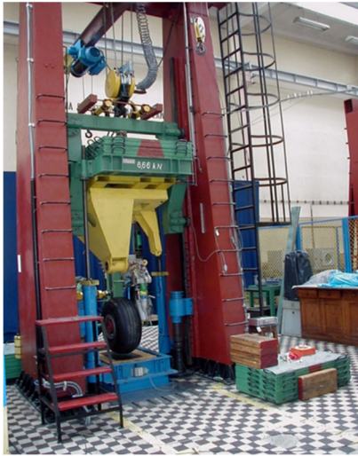
Fig.1. Drop test stand. (source L-Ilot)
