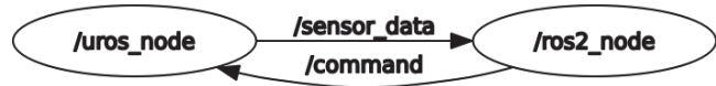
Fig. 9. Rosgraph tool output for application sharing nodes in micro-ROS and ROS 2 systems
