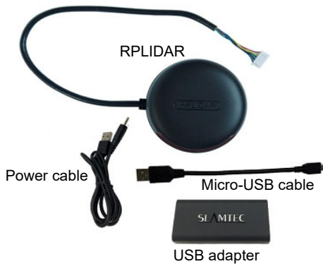
Fig.3. Items in the RPLIDAR Development Kit
