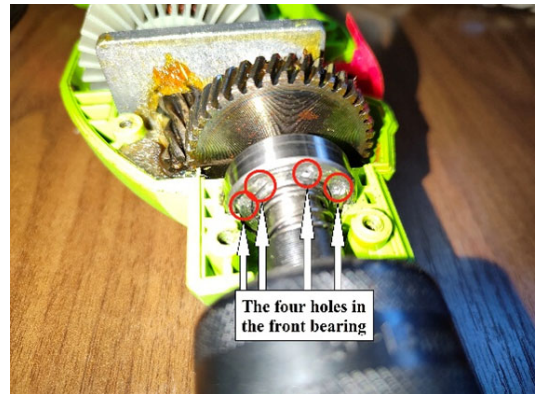
Fig. 3. The impact drill with the four drilled holes in the front bearing.
