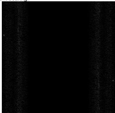
Fig. 15. HCFMwLF image of analyzed impact driller with four drilled holes in front bearing.
