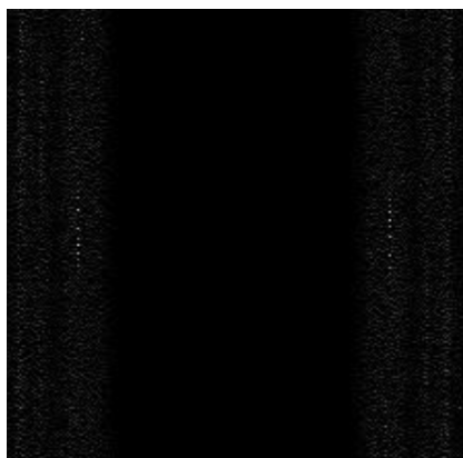
Fig. 23. HCFMwLF image of analyzed impact driller with broken gear.
