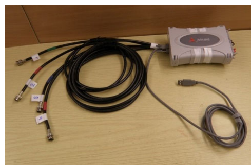
Fig.8. Module for analog-to-digital conversion and data acquisition, of the industrial type USB-1901, enabling the recording of analog signals and the use of a variable number of input channels, with a programmable transmission speed. The manufacturer provides modules with a maximum sampling rate of 250 or 2000 kilosamples per second
