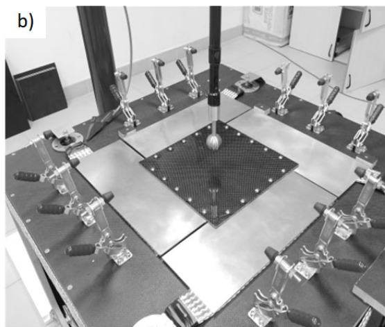
Fig.2. Measurement of current distribution in the sample and voltage drop: a) simplified diagram adopted from [10], b) view of the table with the assembled composite
