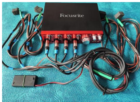
Fig. 1. Device designed and developed by the authors for acoustic emission acquisition of the shoulder joint [13]
