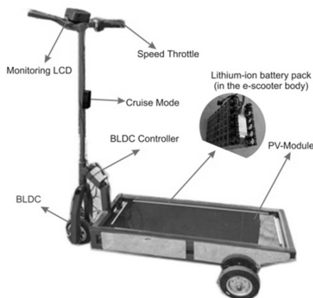
Fig.2. The prototype of solar powered dockless e-scooter (DES)
