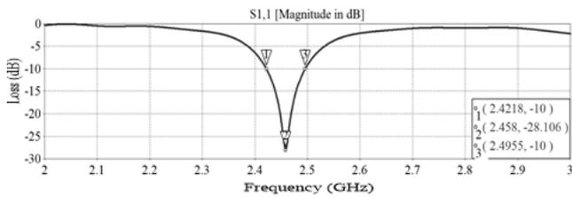
Fig. 5. S11 results for trapezoidal patch antenna
