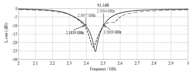
Fig. 10. S11 measurement and simulation results for trapezoidal patch antenna with multi-slot
