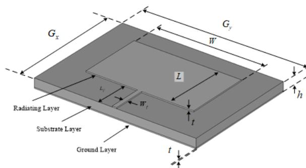
Fig. 1. Regular rectangular patch antenna with microstrip feed.
