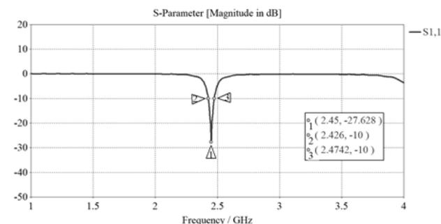
Fig. 2. S11 from simulation results of regular rectangular patch antenna
