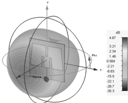
Fig. 7 3D radiation pattern from simulation of the trapezoidal patch with a multi-slot antenna
