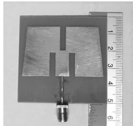
Fig. 9. Trapezoidal patch with multi-slot antenna prototype
