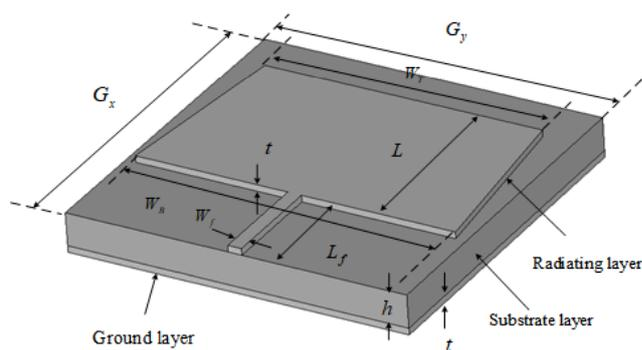
Fig. 4. A trapezoidal patch antenna model
