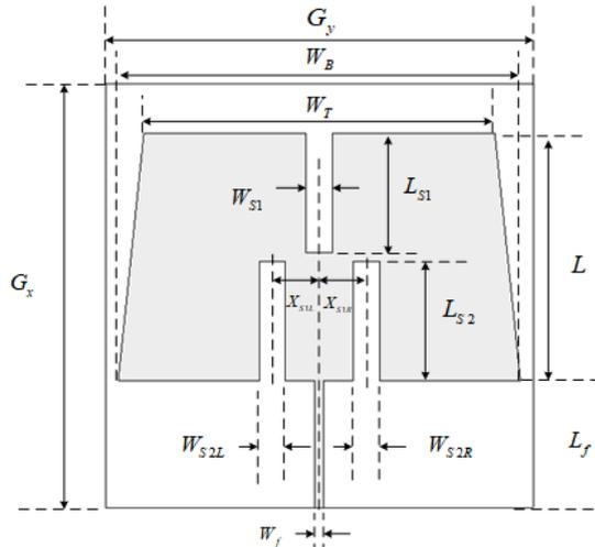
Fig. 6. Model of the trapezoidal patch with the multi-slot antenna
