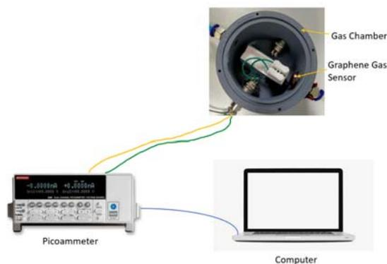
Fig.3. I-V measurement of the gas sensor
