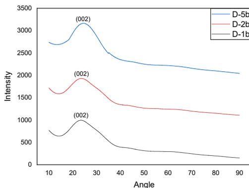
Fig.6. XRD spectra of D-1b, D-2b, and D-5b gas sensors
