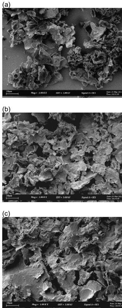
Fig.5. Morphology of the sensing layer of the gas sensor (a) D1b (b) D2b, and (c) D5b
