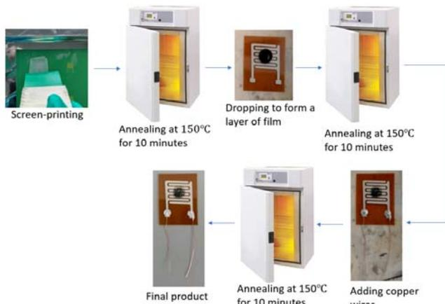
Fig.1. The flow of the gas sensor fabrication process
