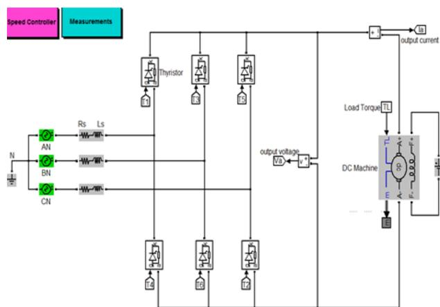
Fig. 2. The second proposed power system of the DCM drive circuit
