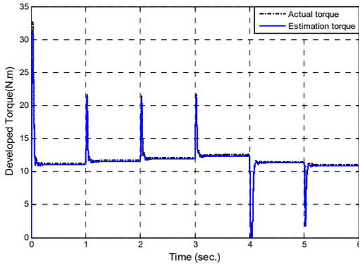
Fig. 9. Electrical developed torque responses of the second suggested circuit at different speed and constant load torque.
