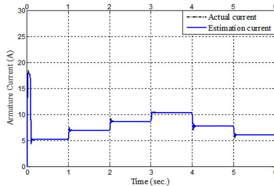
Fig. 16. Armature voltage and current responses of the SDCM .
