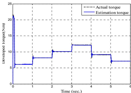
Fig. 14. Electrical developed torque responses of the SDCM under various load torque and constant speed for the first circuit
