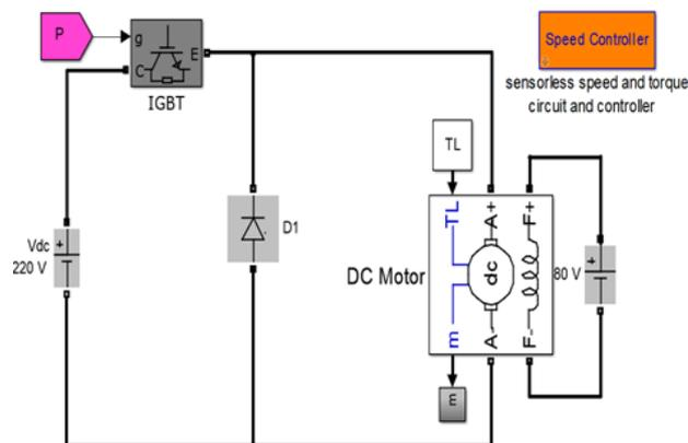
Fig. 1. The first proposed power system of the DCM drive circuit.
