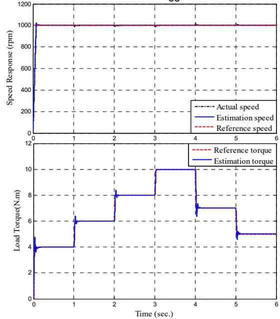
Fig. 12. Speed/torque response of the SDCM for the first model
