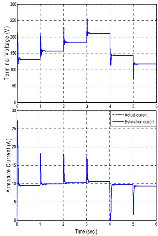
Fig. 11. Terminal armature voltage and current responses of the SDCM for the second suggested circuit
