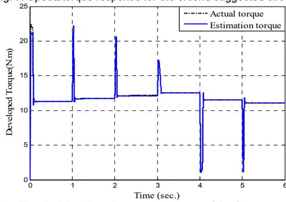
Fig. 8. Electrical developed torque responses of the first suggested circuit at different speed and constant load torque.
