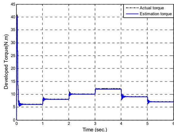
Fig. 15. Electrical developed torque responses of the SDCM under various load torque and constant speed for the second circuit
