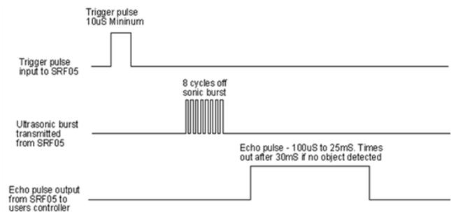
Fig. 8 Ultrasonic (SRF05) signals [20]
