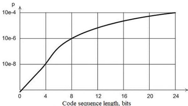
Fig. 10. Probability of an irreparable error depending on the length of the informational message
