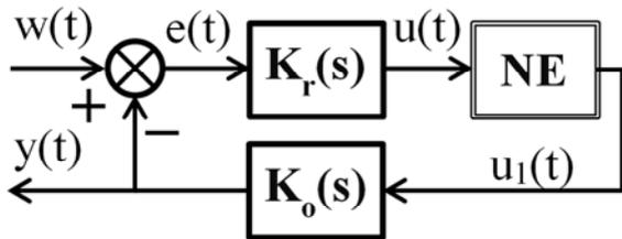
Fig.3. Block scheme of the considered control system with nonlinear element – saturation
