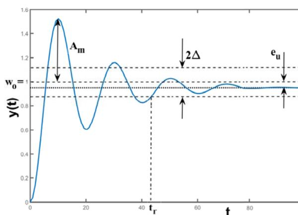
Fig.2. Output signal  $y(t)$  with marked parameters  $A_m$ ,  $t_r$ , and  $e_u$
