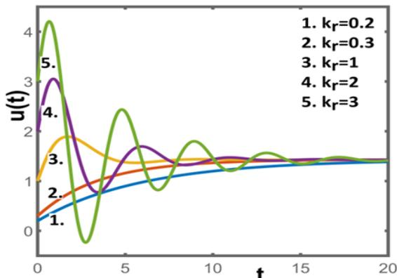
Fig.9. Control signal  $u(t)$  for various values of  $k_r$ .
