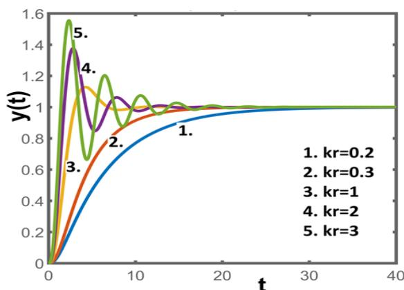
Fig.8. Output signal  $y(t)$  for various values of  $k_r$  for example 2
