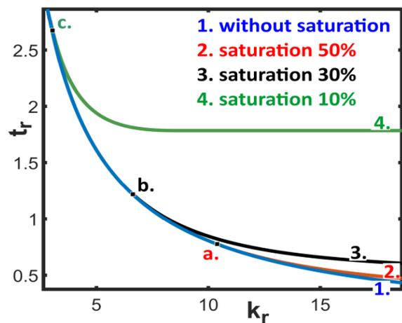
Fig.5. The dependence of the settling time  $t_r$  on  $k_r$  for control systems with and without saturation
