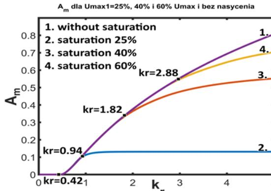
Fig.11. The dependence of the overshoot  $A_m$  on  $k_r$  for control systems with and without saturation
