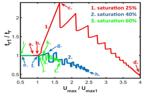
Fig.12. Relative control quality indicator for  $t_r$  for saturation  $U_{max1}=25\%U_{max}$ ,  $U_{max1}=40\%U_{max}$  and  $U_{max1}=60\%U_{max}$
