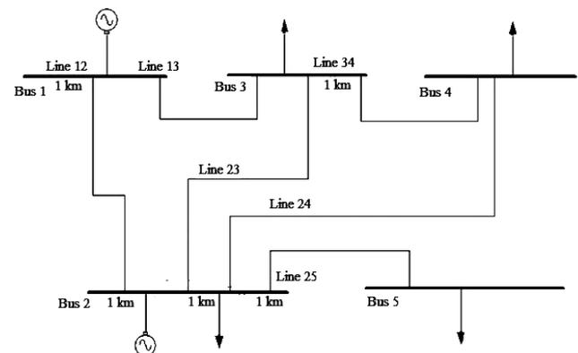
Fig. 10. The 5-bus system layout under line 4-5 outage
