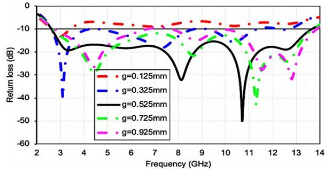
Fig. 6. Predicated return loss arcs with diverse numbers of g parameter.
