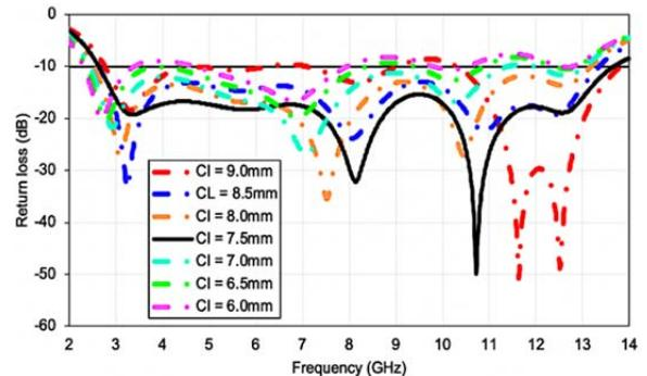
Fig. 2. Predicated return loss arcs with various numbers of  $Cl$  parameter
