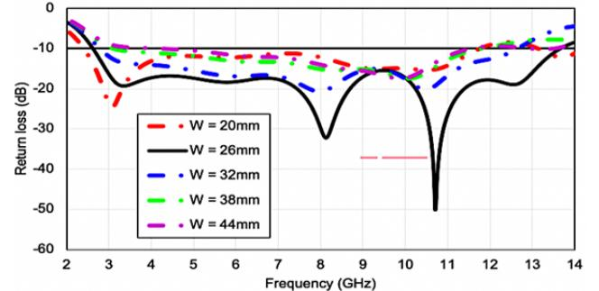
Fig. 4. Predicated return loss arcs with various numbers of  $W$  parameter
