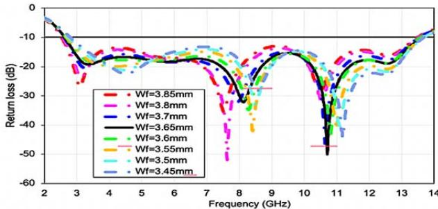
Fig. 5. Simulated return loss curves with different numbers of Wf parameter
