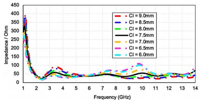
Fig. 3. Simulated input impedance for different numbers of  $Cl$  parameter
