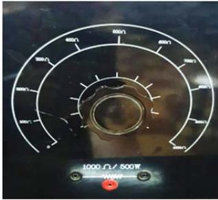
Fig.8. Series armature control resistances.
