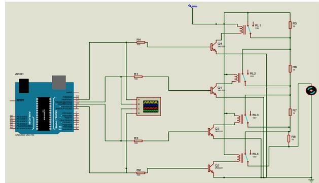
Fig.11. Proteus simulation for speed control of series DC motor.
