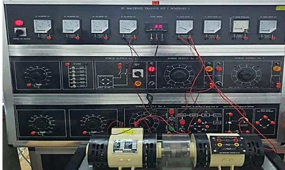
Fig.12. Controlling the speed of a DC series motor with a practical circuit.
