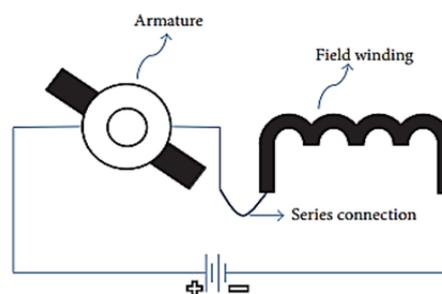
Fig.1. DC series motor connection
