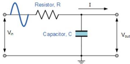
Fig 6. Filter Circuit
