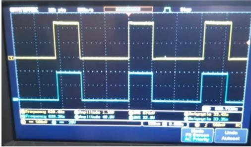
Fig 14. Comparison of Microcontroller and IR2104 . High Side Signals
