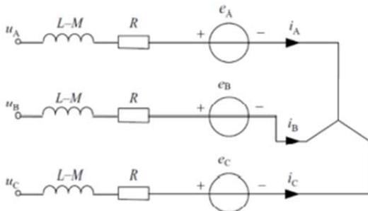
Fig 1. BLDC motor equivalent circuit
