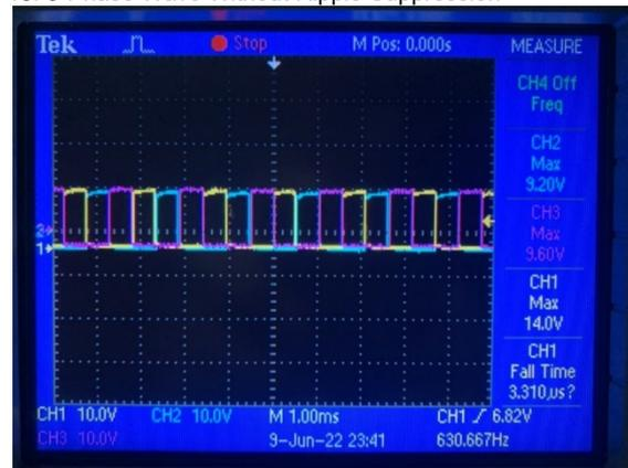
Fig 19. 3-Phase Wave With Ripple Suppression
