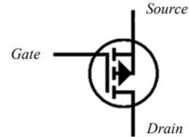
Fig 2. MOSFET Circuit
