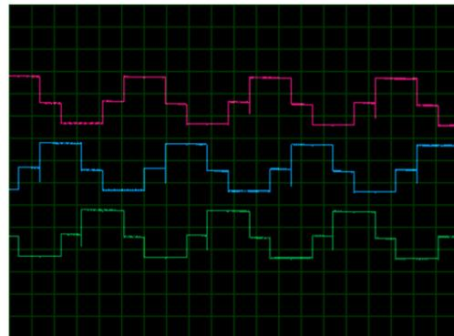
Fig 13. Back-Emf Simulation Results
