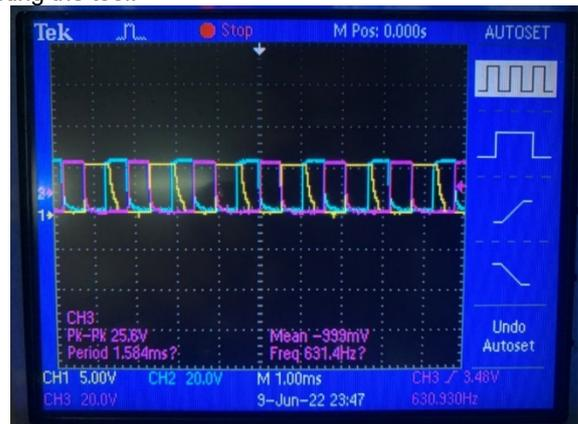
Fig 18. 3-Phase Wave Without Ripple Suppression
