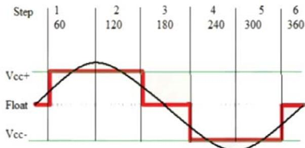
Fig 5. Determination of the Six-Step Method
