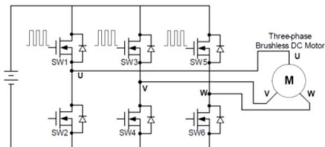
Fig 3. 3 Phase Inverter Circuit
