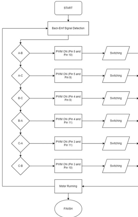
Fig 9. Six-Step Commutation Switching Logic
