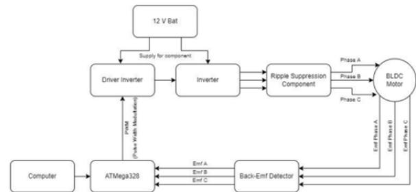
Fig 7. Control Circuit System Schematic
