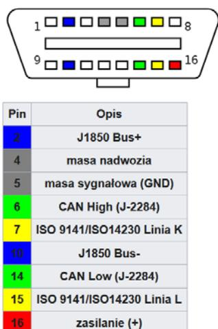
Fig. 5. Diagram of the OBDII system connector [10].
