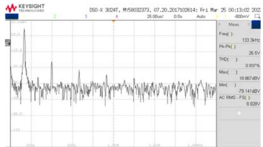
Fig.12. The frequency of the LC oscillator with the caprio technique, number of inductance L3 = 20 turns.
