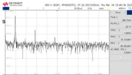
Fig.7. The frequency of the LC oscillator with the caprio technique, number of inductance L3 = 5 turns.
