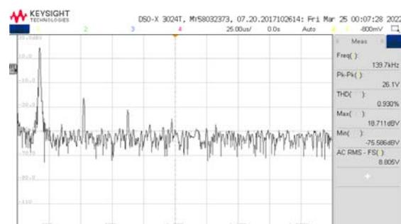
Fig.11. The frequency of the LC oscillator with the caprio technique, number of inductance turns L3 = 17
