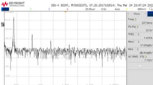
Fig.8. The frequency of the LC oscillator with the caprio technique, number of inductance L3 = 7 turns.
