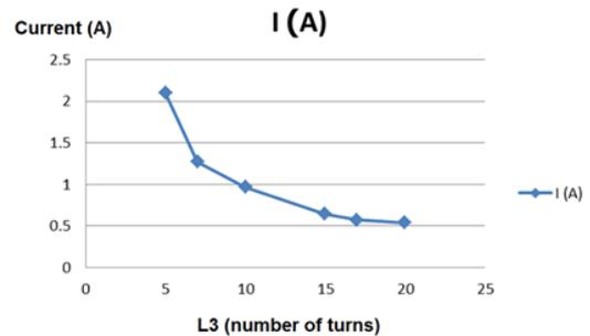
Fig.13. The current of the LC oscillator using the caprio technique when varying L3
