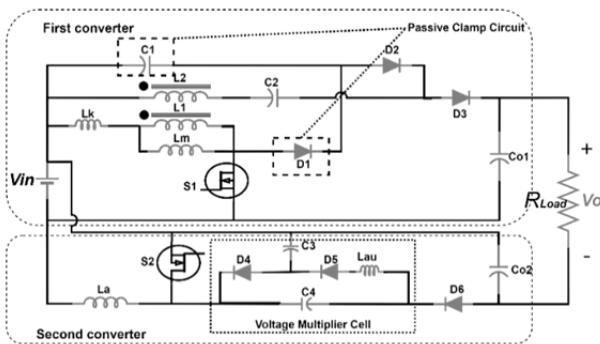
Fig. 1. The schematic graph of the proposed converter
