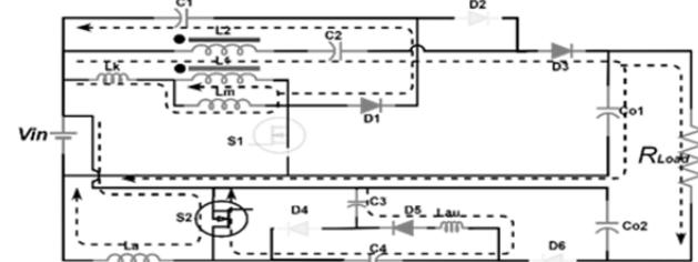
Fig 5. Equivalent circuits in mode 5
