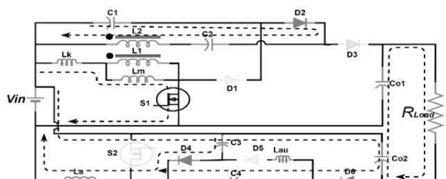
Fig 4. Equivalent circuits in mode 3
