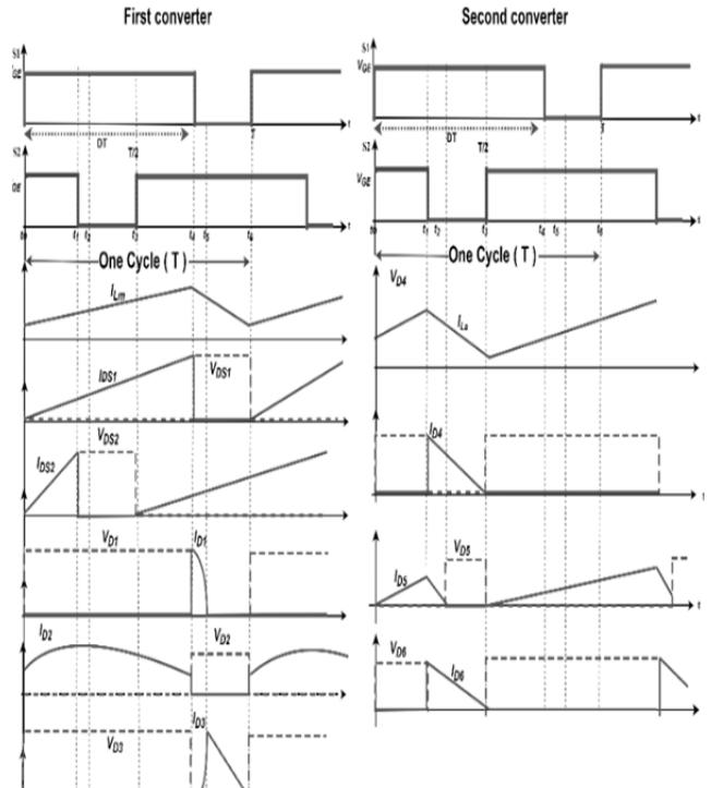
Fig 7. The sample waveforms of the proposed converter under steady-state operation.
