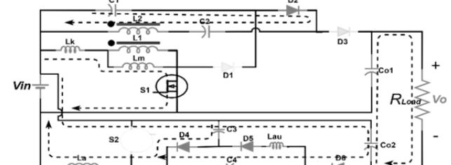
Fig 3. Equivalent circuits in mode 2
