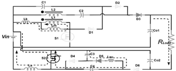
Fig 6. Equivalent circuits in mode 6
