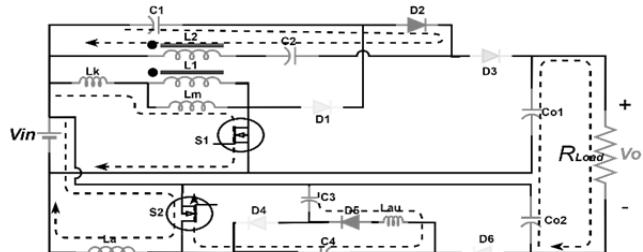
Fig 2. Equivalent circuits in mode 1&mode 4
