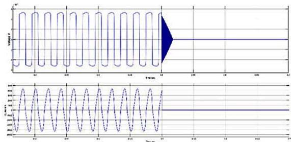
Fig. 5. Voltage and current waveforms vs time at MOV1 waveforms at MOV2.
