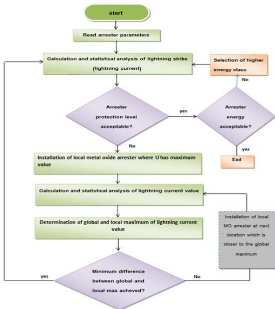
Fig. 4. Flowchart of lightning metal oxide surge arrester on T.L
