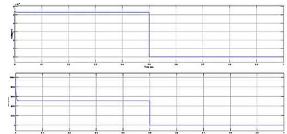
Fig. 12. Voltage and current waveforms vs time at MOV2.
