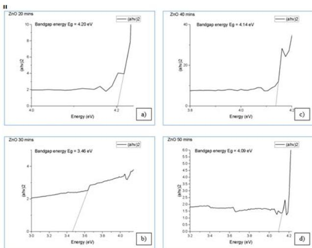
Fig. 6: Bandgap of deposited ZnO thin film on ITO glass with different the deposition times; a) 20 minutes, b) 30 minutes, c) 40 minutes, and d) 50 minutes.
