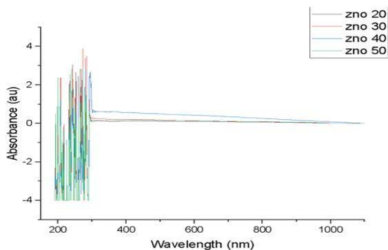
Fig. 5: Absorption spectra of ZnO thin film with different deposition time (20, 30, 40 and 50 minutes with fix molarity of 0.01M).
