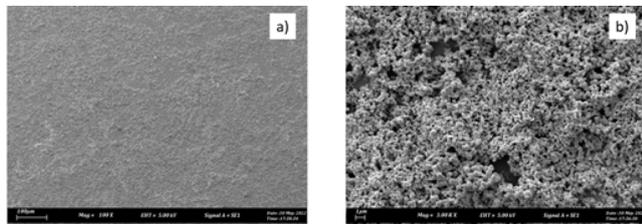
Fig. 12: The ZnO thin film deposited under deposition potentials of -0.61V with the molarity, 0.1M at 30 minutes of deposition time; a) magnification of 100 and b) magnification of 3000.
