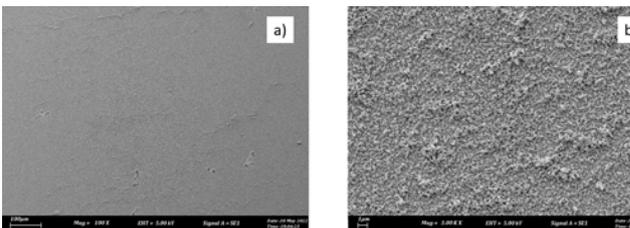
Fig. 10: The ZnO thin film deposited under deposition potentials of -0.61V with the molarity, 0.01M at 30 minutes of deposition time; a) magnification of 100 and b) magnification of 3000.
