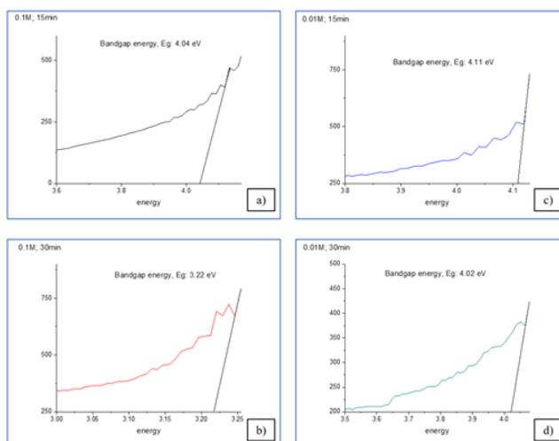
Fig. 8: Bandgap of deposited ZnO thin film on ITO glass with different in molarity and deposition times; a) 0.1M and 15 minutes, b) 0.1M and 30 minutes, c) 0.01M and 15 minutes, and d) 0.01M and 30 minutes.
