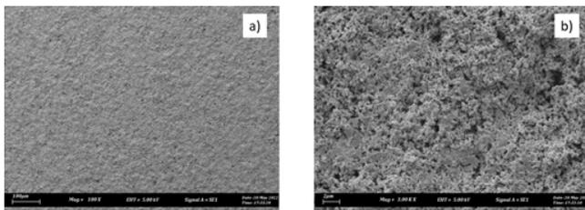
Fig. 11: The ZnO thin film deposited under deposition potentials of -0.61V with the molarity, 0.1M at 15 minutes of deposition time; a) magnification of 100 and b) magnification of 3000.
