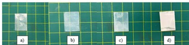
Fig. 4: The ZnO was deposited for a) 15 minutes and 0.01M, b) 30 minutes and 0.01M, c) 15 minutes and 0.1M, and d) 30 minutes and 0.1M, respectively, under deposition potentials of -0.61V at 90°C and pH value of 5.74.
