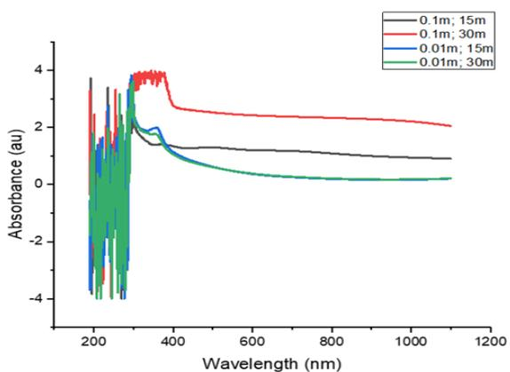
Fig. 7: Absorption spectra of ZnO thin film with different deposition times (15 and 30 minutes) for each molarity of 0.01 and 0.1 M.
