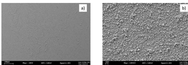
Fig. 9: The ZnO thin film deposited under deposition potentials of -0.61V with the molarity, 0.01M at 15 minutes of deposition time; a) magnification of 500 and b) magnification of 3000.
