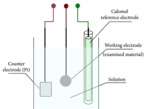
Fig. 2: The illustration of the three-electrode setup for electrodeposition process.
