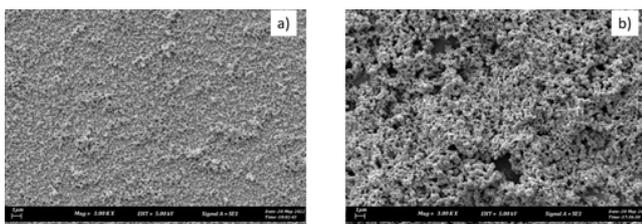
Fig. 13: Comparison of the electrodeposited thin film ZnO using aqueous solution of 0.01M and 0.1M in 30 minutes.
