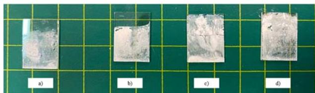
Fig. 3: The ZnO was deposited for a) 20 minutes, b) 30 minutes, c) 40 minutes, and d) 50 minutes, respectively, under deposition potentials of -0.61V at 90°C and pH value of 5.74.
