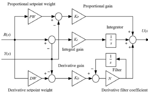
Fig.2. Two degrees of freedom (2-DOF) PIDcontroller
