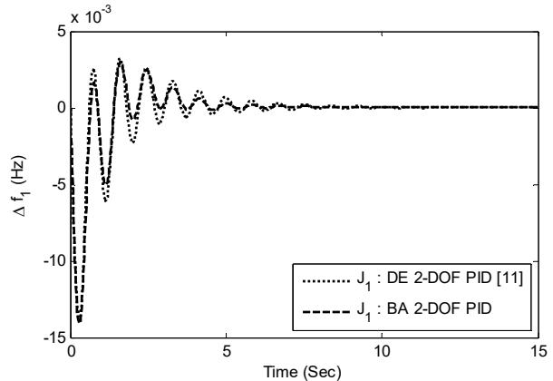
Fig.3. Frequency deviation of area-1 for 1% change in area-1 with ISE objective function.
