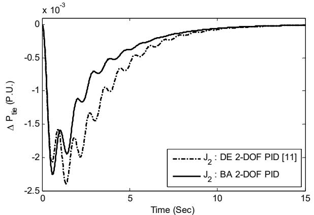
Fig.8. Tie line power deviation for 1% change in area-1 with ITSE objective function.
