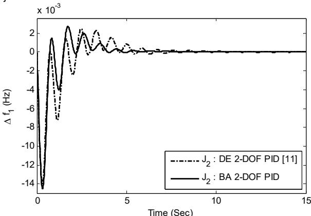
Fig.6. Frequency deviation of area-1 for 1% change in area-1 with ITSE objective function.
