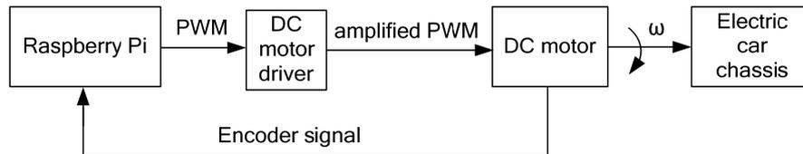
Fig. 1. Functional chart of the laboratory set-up
