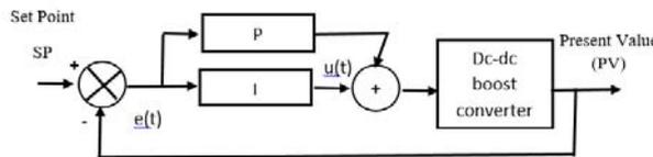
Fig 3. The PI Control System
