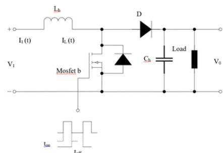
Fig 1. Circuit of DC-DC Boost Converter
