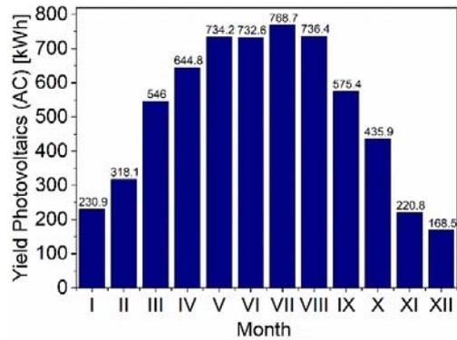
Fig. 7 The monthly electricity production AC by the PV solar system
