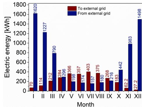
Fig. 8 Electric energy withdrawn to and from the external power grid
