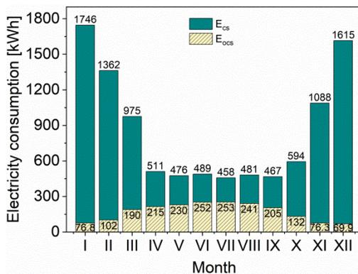
Fig. 6 Self-consumption (E<sub>OCS</sub>) and total electricity consumption (E<sub>CS</sub>) by month
