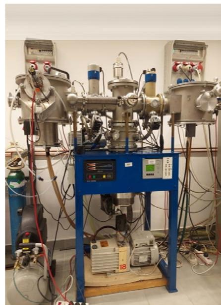
Fig. 1. Picture of the magnetron deposition equipment with two vacuum chamber
