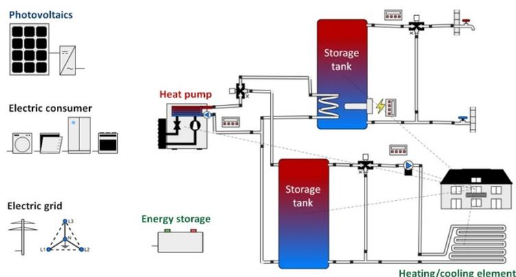
Fig. 3 Model of energy system consisting of photovoltaic modules, energy storage and heat pump applied to simulation by using the Vela Solaris Polysun
