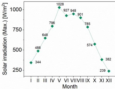
Fig. 5 Maximum solar irradiance by month of the year for Krakow (Poland) output from Polysun software
