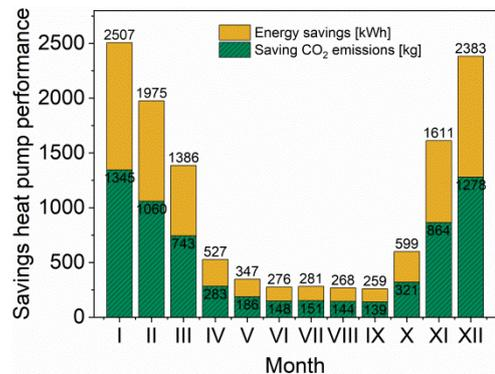
Fig. 9 The energy and CO<sub>2</sub> savings due to the heat pump performance factor, compared to electric resistance heating system
